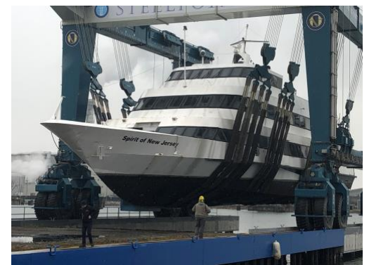
700-ton Marine Travelift Well at Bridgeport Boatworks
